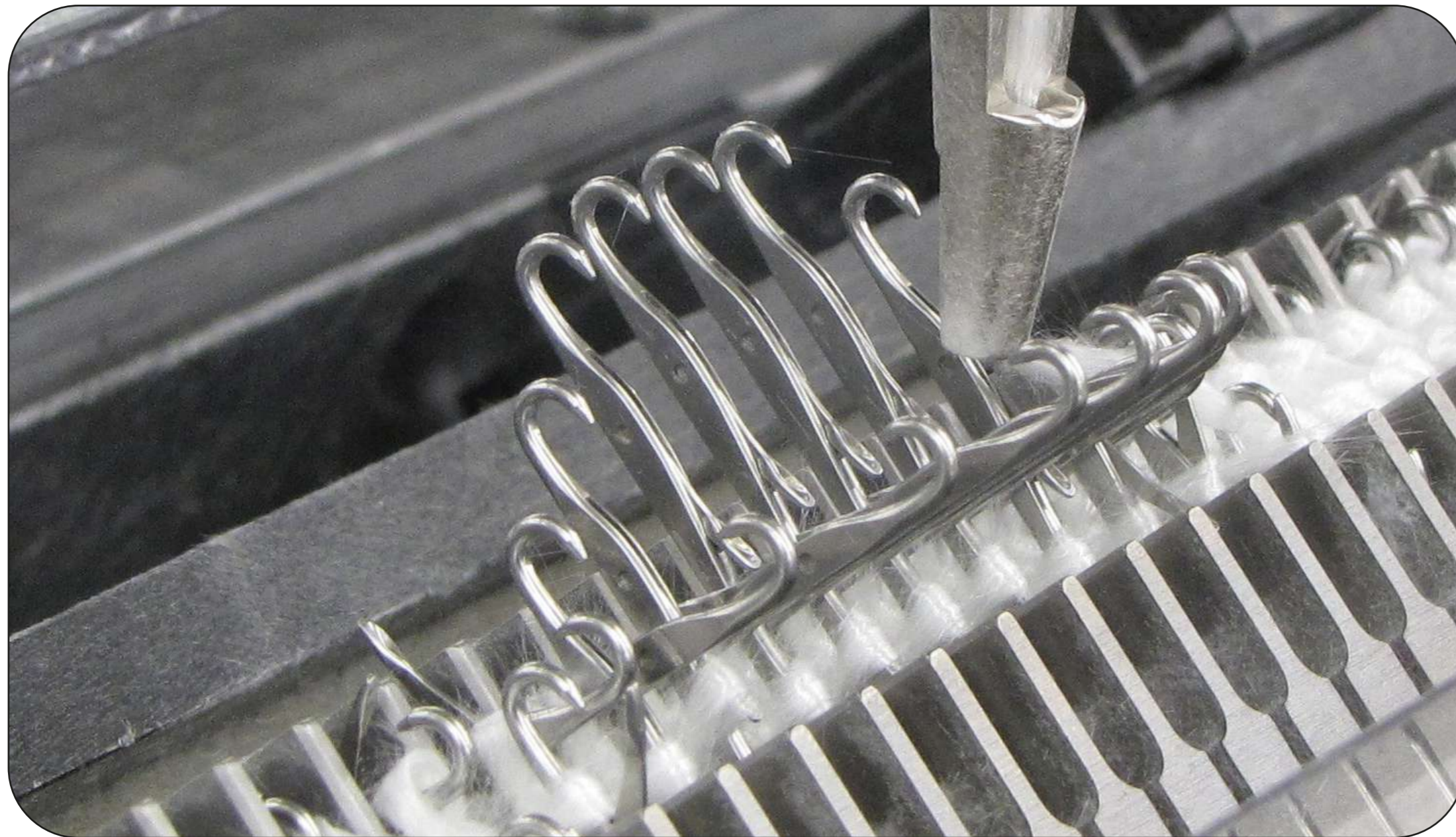
Fig: Knitting is the method of creating fabric by transforming continuous strands of yarn into a series of interlocking loops.
